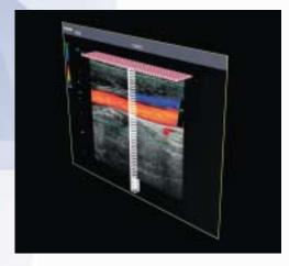
Continuously thin ultrasonic beam of a Matrix Transducer due to Dynamic Micro Slice technology.
