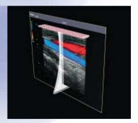
Variable slice thickness in one-dimensional transducers due to lens focusing in elevation direction.
