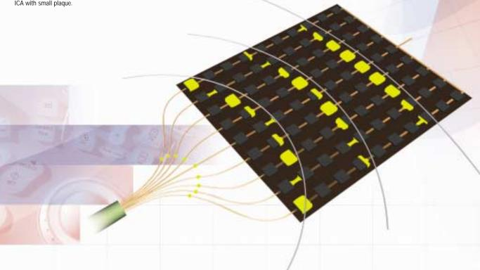
The key to the Tera Processing Beamformer's accuracy lies in dedicated processing channels for each individual transducer element. The system calculates the optimum delay pattern realtime for each element at each depth. And processing channels can be individually adapted dynamically to current scanning conditions. This unique technology produces a continuous thin beam with focal point uniformity over all depths resulting in excellent sensitivity and resolution.
